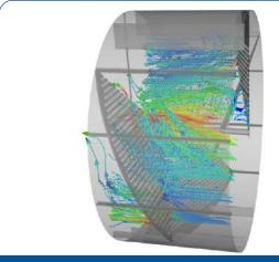
The patented HELIXCHANGER baffle construction is backed up by laboratory test data, state of the art computational fluid dynamics (CFD) and extensive field data.
