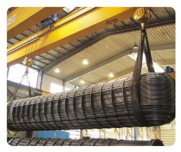
The HELIXCHANGER® heat exchanger uses Lummus Technology's industry proven, enhanced heat transfer technology to provide solutions for common issues such as shell-side fouling, high pressure drop and vibration. It is a particularly efficient choice for expansions or plant upgrades with lean budgets and limited plot space.
